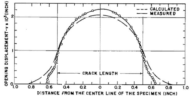
Fig. 4—Opening displacement along crack line:  $\sigma$ , 55 ksi;  $\sigma_Y$ , 91 ksi;  $E$ ,  $32 \times 10^6$  psi; thickness, 0.012 in.; width, 6 in.; slot length, 1.0 in.
