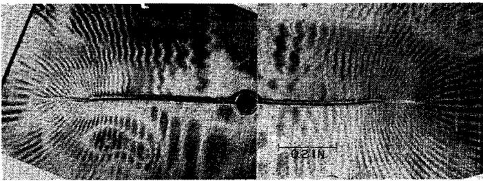
Fig. 1—Moiré pattern of a steel specimen: applied stress, 55 ksi; 0.2-percent-offset yield stress, 91 ksi; Young's modulus,  $32 \times 10^6$  psi; 0.012-in. thick; 6-in. wide; slot length, 1.0 in.; pitch of moiré grille,  $1/13,400$  in.
