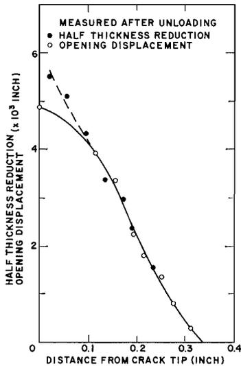
Fig. 8—Half-thickness reduction and opening displacement in the strip necking region of a steel specimen.  $\sigma$ , 62 ksi
