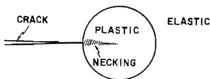
Fig. 6—Schematic diagram of the various regions of deformation around a crack
