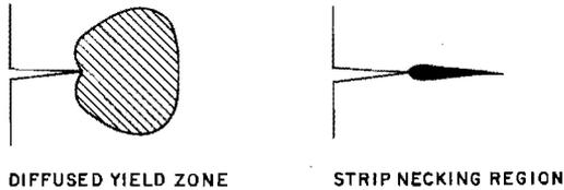
Fig. 2—Schematic diagrams of diffused yield zone and strip necking region
