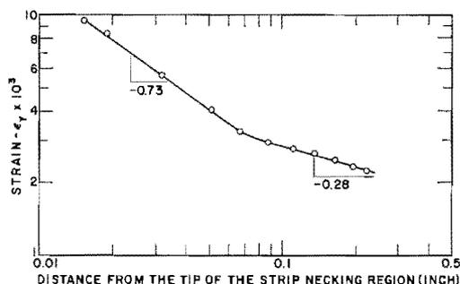
Fig. 5—Strain ahead of the strip necking region
